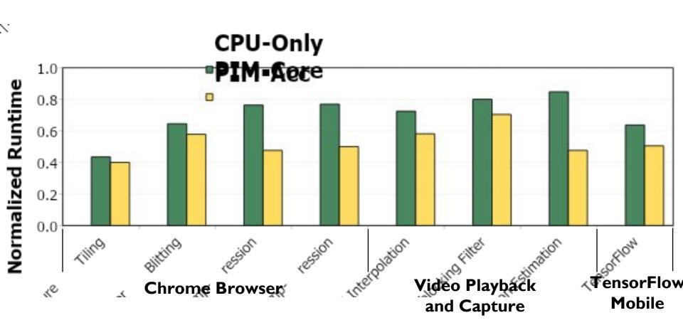
Offloading these kernels to PIM core and PIM accelerator improves performance on average by 44.6% and 54.2%
