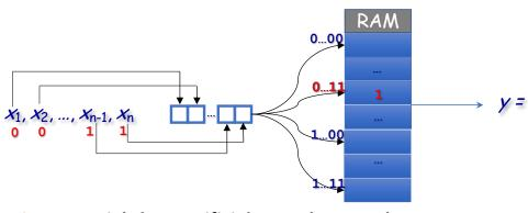
N-tuple sampling machine Bledsoe and Browning, 1959
