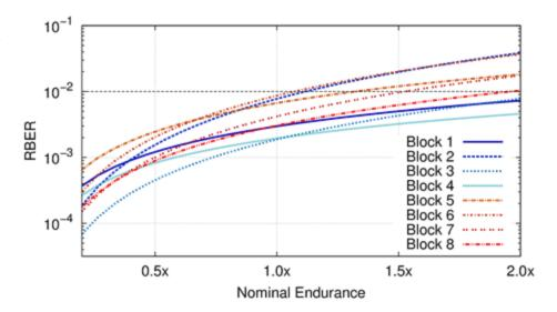
RBER of different flash blocks in the same device as a function of P/E cycles
