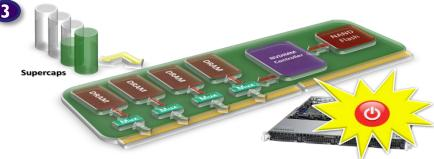
• During unexpected power loss event, DRAM contents are moved to NAND Flash using Supercaps for backup power
