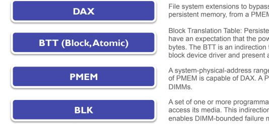
File system extensions to bypass the page cache and block layer to memory map persistent memory, from a PMEM block device, directly into a process address space.
