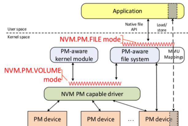
SAP HANA focus is on leveraging memory mapping in NVM.PM.FILE mode which enables direct access to persistent memory using CPU instructions
