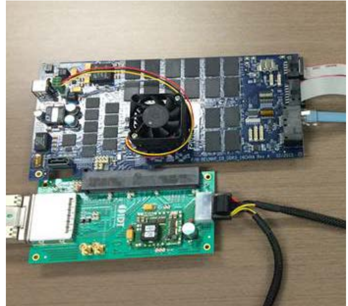
The PMC Flashtec evaluation card with Micron NAND and DDR. No ReRAM attached (yet) unfortunately ;-).
