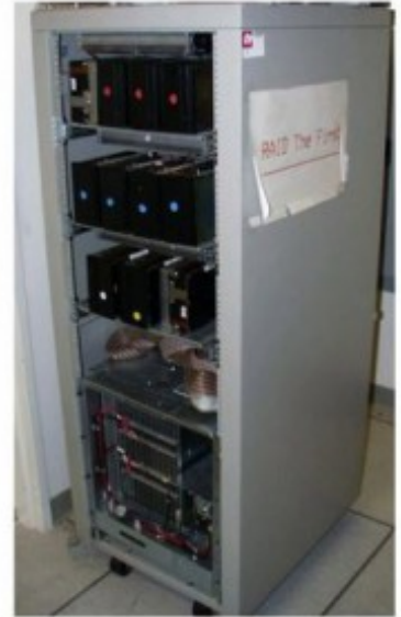
RAID1 (1989) - Sun 4/280 WS, 128 MB DRAM, 4 dual-string SCSI controllers, 28 5.25-inch SCSI disks with disk mirroring software
