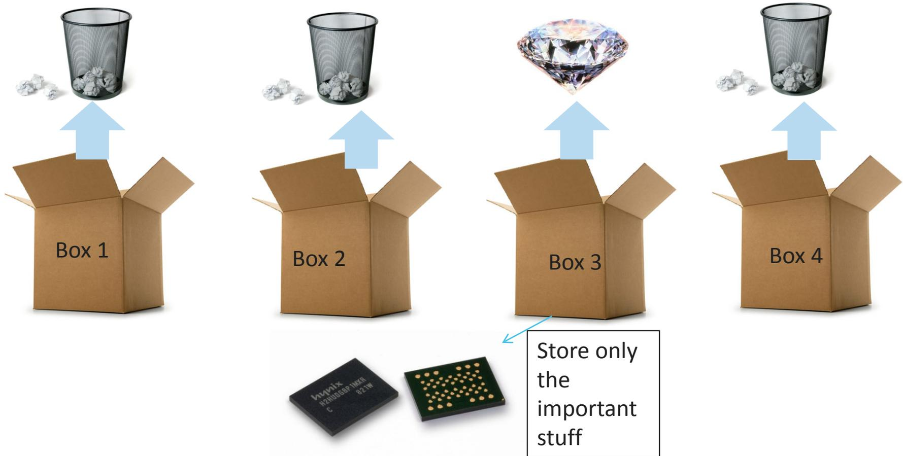
Driver based solutions look inside of the box and places the most important information into the NAND subsystem, which should eventually lead to either endurance or speed advantages. Because of this insight, the SATA-IO standards group to created a hinting protocol to help do intelligent caching.
