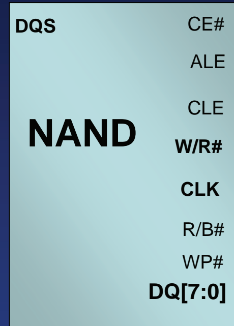
Source Synchronous NAND Interface
