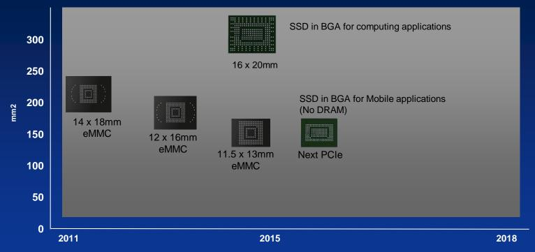
DRAM-less PCIe/NVMe SSDs can be packaged in 11.5 x 13mm
