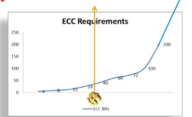
ECC Bits = F (WA, Target Life Span, Target UBER, Type of Material, ...)
